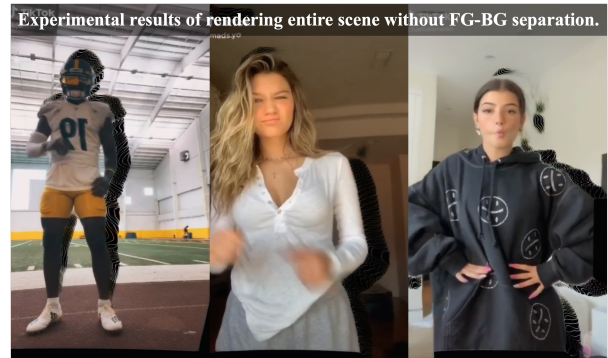
Fig. 12. Ablation study on foreground-background separation. Unified rendering without separation leads to severe geometric distortions and artifacts during viewpoint changes due to differing depth structures. In contrast, our method models them as separate point clouds to preserve depth ordering and ensure stable rendering under simultaneous motion and camera transformation.
