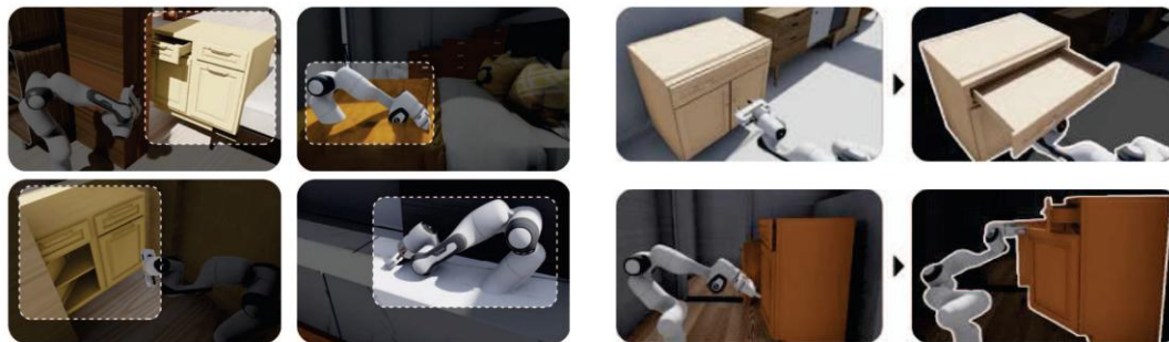
(a) Improper room layout causing inaccessibility or collision
