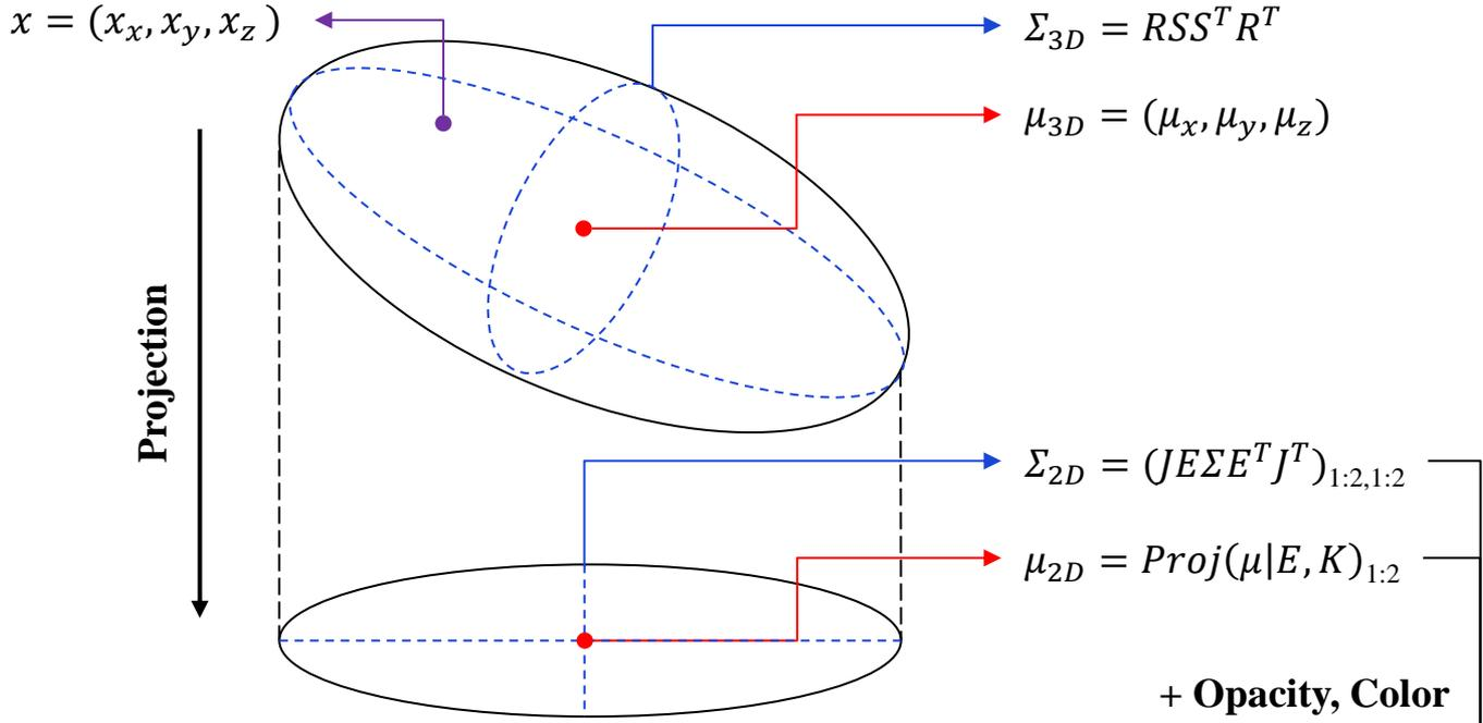
$$I(u, v) = \sum_{i=1}^N p_i(u, v; \boldsymbol{\mu}_{2D}, \boldsymbol{\Sigma}_{2D}) \alpha_i c_i(d_i) \prod_{j=1}^{i-1} (1 - p_j(u, v; \boldsymbol{\mu}_{2D}, \boldsymbol{\Sigma}_{2D}) \alpha_j)$$
