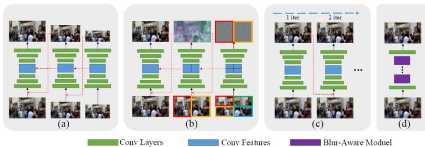
Figure 2. Comparison of coarse-to-fine image deblurring network architectures: (a) DeepDeblur, (b) PSS-NSC, (c) MT-RNN, and (d) proposed MIMO-UNet.
